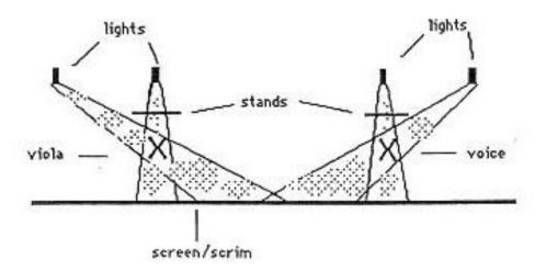
Two lights should be focused on each performer (see diagram), the lighting should take care to facilitate the greatest possible amount of interaction among the projected images.
